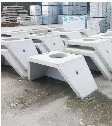
Wing walls in SVC yard.
