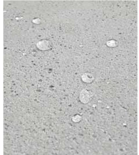
This concrete surface was sealed with a penetrating sealer, rendering it water-resistant.
