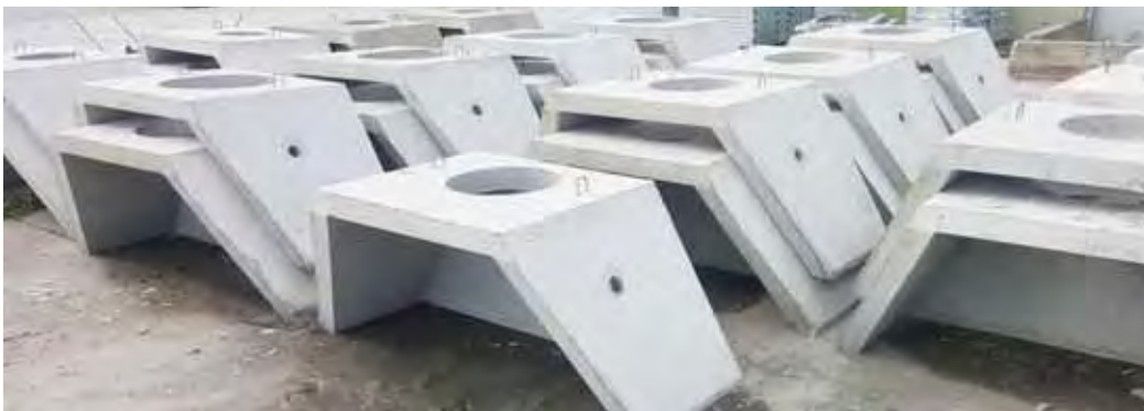
Wingwalls act as retaining walls and allow pipes to be passed through.
